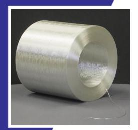
FGOC ECPlus Direct Roving 621 is produced with ECPlus boron free glass consisting of continuous glass fibers manufactured by the direct draw process and winding them on cylindrical package. The roving is treated with a special sizing system based on silanes which provides excellent performance with a wide variety of thermoset resins such as polyester, vinyl ester, epoxy etc. These rovings are designed to be used in filament winding, pultrusion and weaving processes and provide:
